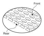
Note: The grill has a front and rear, the holes on the front side have rounded edges and the rear holes have flat edges.
